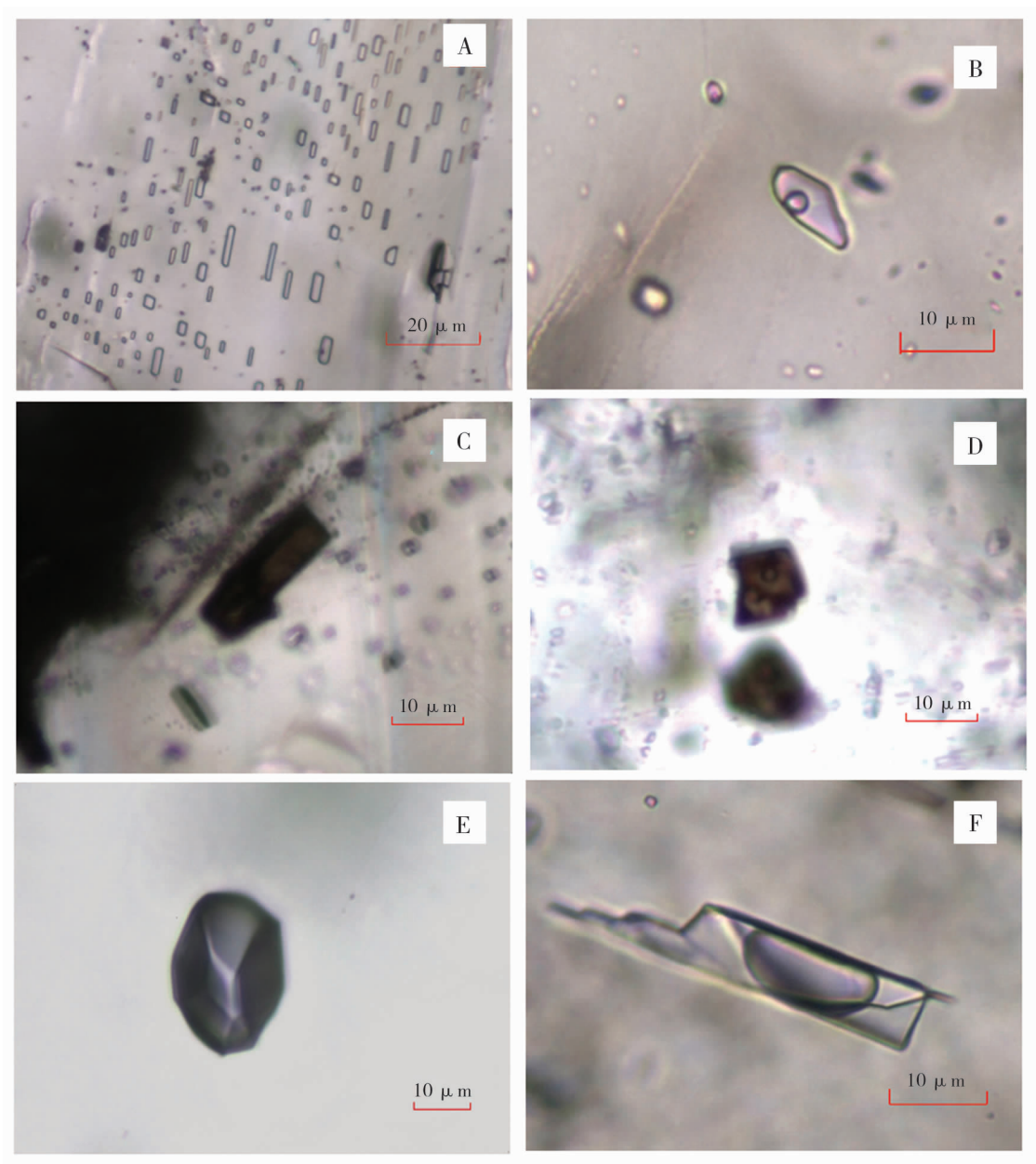
A-液相水包裹体(普光6井,PG6-69);B-气液水包裹体(普光9井,PG9-23);C-含沥青液相烃包裹体(普光9井,PG9-22); D-含沥青气液烃包裹体(偏岩子,PY-11);E-气相烃包裹体(普光6井,PG6-69);F-烃-水包裹体(普光9井,PG9-24) A-liquid water inclusions; B-gas-liquid water inclusions; C-including asphalt liquid hydrocarbon inclusions; D-including asphalt gas-liquid hydrocarbon inclusions; E-gas phase hydrocarbon inclusions; F-hydrocarbon-water inclusions
